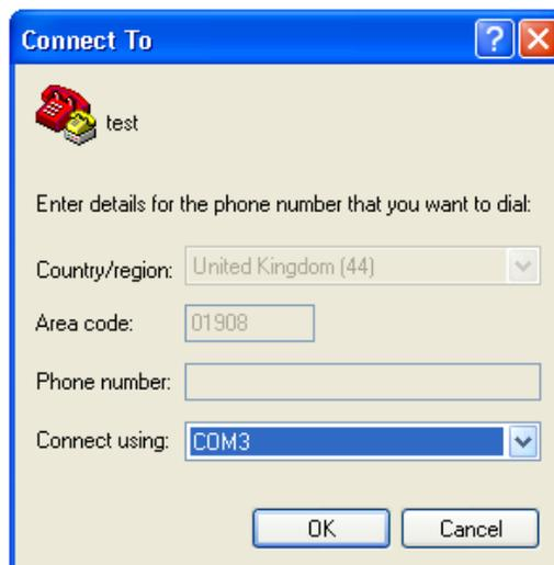
Set the com port to the virtual com port of your USB to RS232 convertor – COM3 in this example. Next set the Baud settings, typically 4800 Bps, 8 data bits, no parity and 1 stop bit for most ADAM scales (though not all, so you need to check the user manual’s RS232 Section to find out how to check the settings inside your scale/balance.
